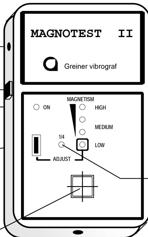
Press and it will divide the reading by 4. Use when object has strong magnetic reading
